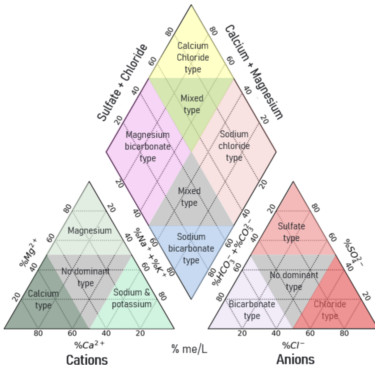
Exhibit 1. Piper diagram components – bottom left is a ternary plot of the cations, bottom right is a ternary plot of the anions, and top is a diamond plot of a project from the other two plots.
