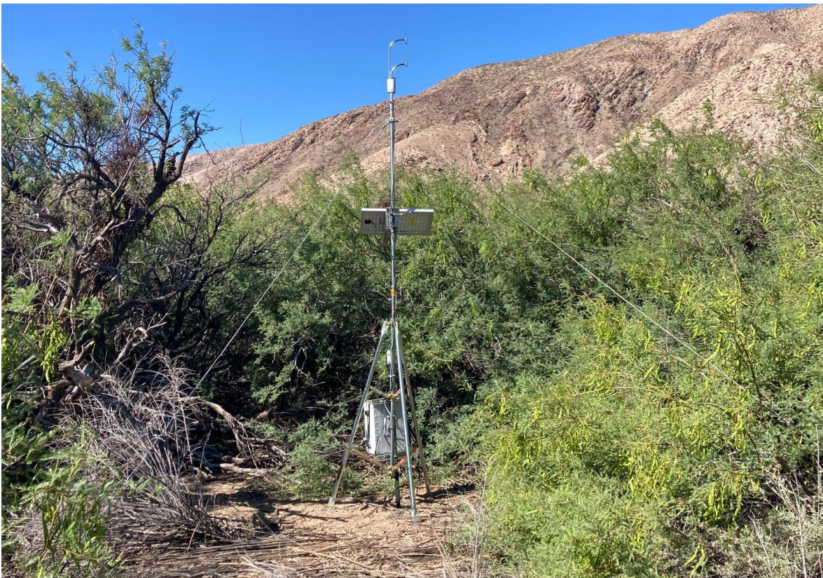
Figure 5. The LI-COR LI-710 evapotranspiration (ET) sensor measures evapotranspiration by detecting water vapor released from plants and soil, offering real-time insights into the amount of water being transferred from the ecosystem to the atmosphere. Above is an image of the instrument located in the mesquite bosque habitat at Clark Dry Lake.
